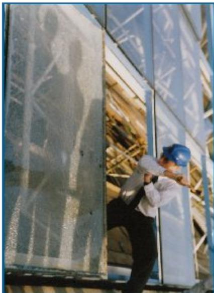
Clear safety film is designed to hold shattered glass in place when broken.
